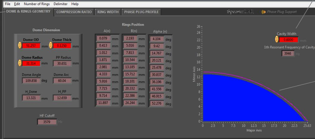
**Cavity width** is the volume area between Dome and Phase Plug. In other words, this gap is the distance between the inner diameter of the dome and the outer diameter of phase plug.
