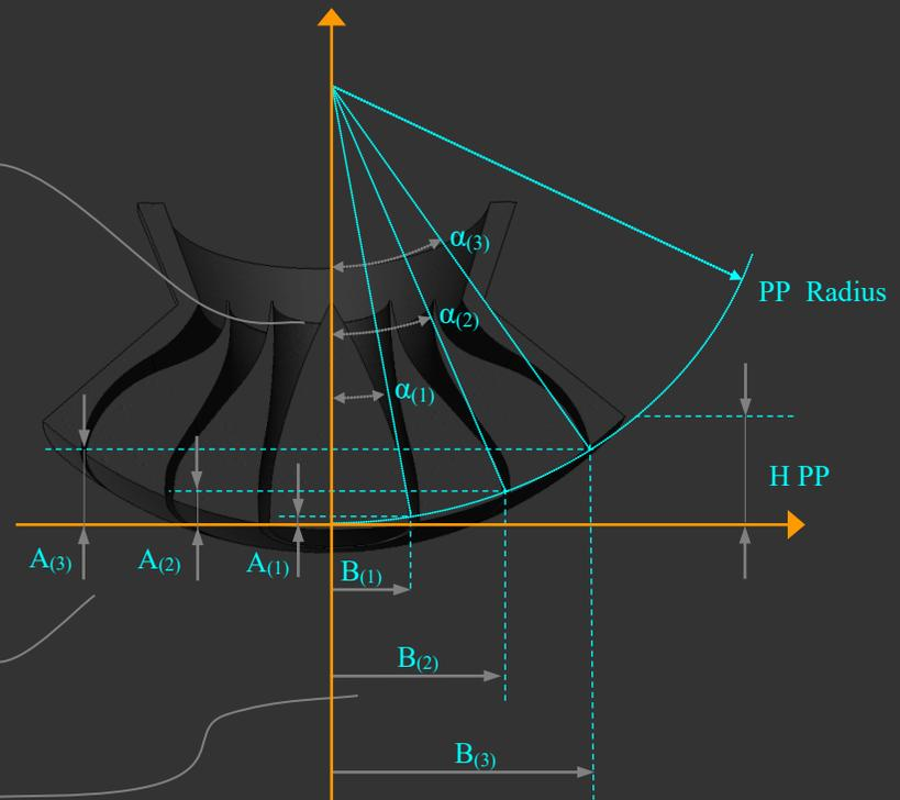
Moving yellow point **cursor** is possible to set the required **Phase Plug Length**. By this way the designer has the channels path on left side and the compression driver exit on right side (usually integrated in the pole plate). Positioning the cursor on maximum path length it's possible to design a full path phase plug.
