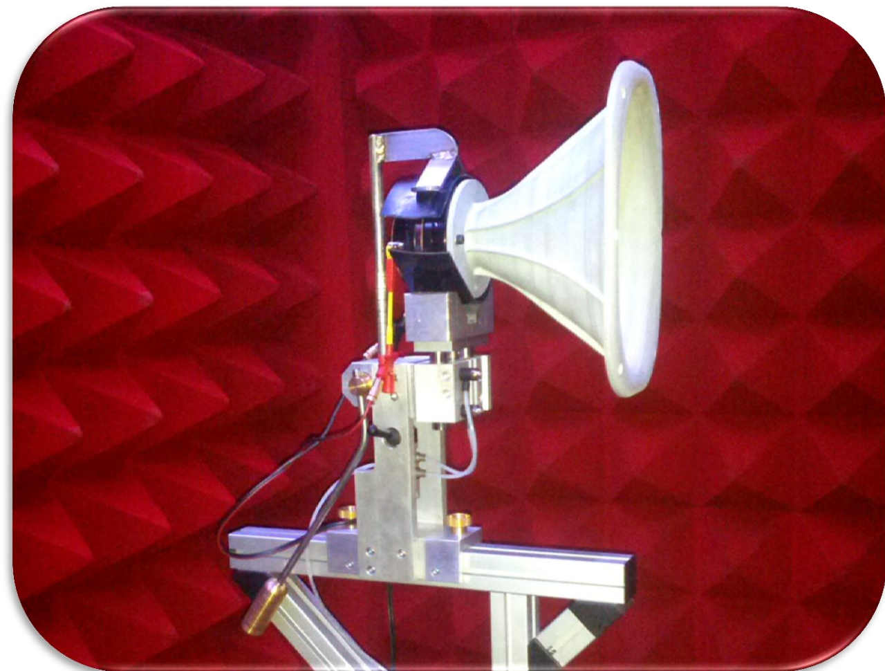
Measuring real objects in anechoic room with the horn fast prototype
