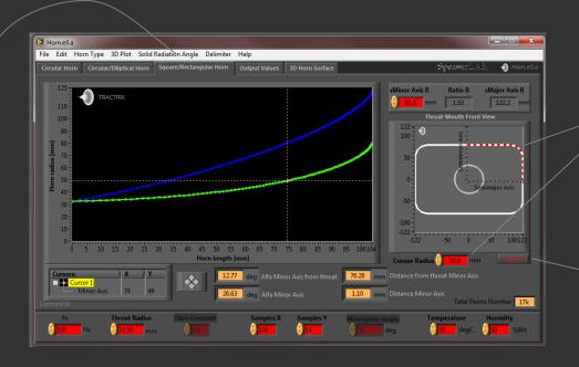
Increasing the value of Corner Radius, it reduces sharp edges along the acoustical path inside the horn.
