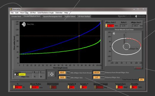
In the **Horn Mouth** graph there is the mouth representation. In the **upper box** is possible to edit s**Minor Axis** value to give the required aspect ratio of the mouth shape. Aspect Ratio is an indicator of the horizontal and vertical coverage angle.
