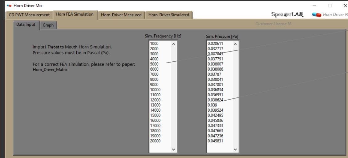
Paste the frequency column (in Hz)
