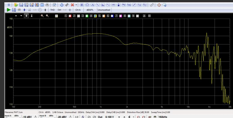
Suggested PWT measurement: sinusoidal sweep signal @1W
