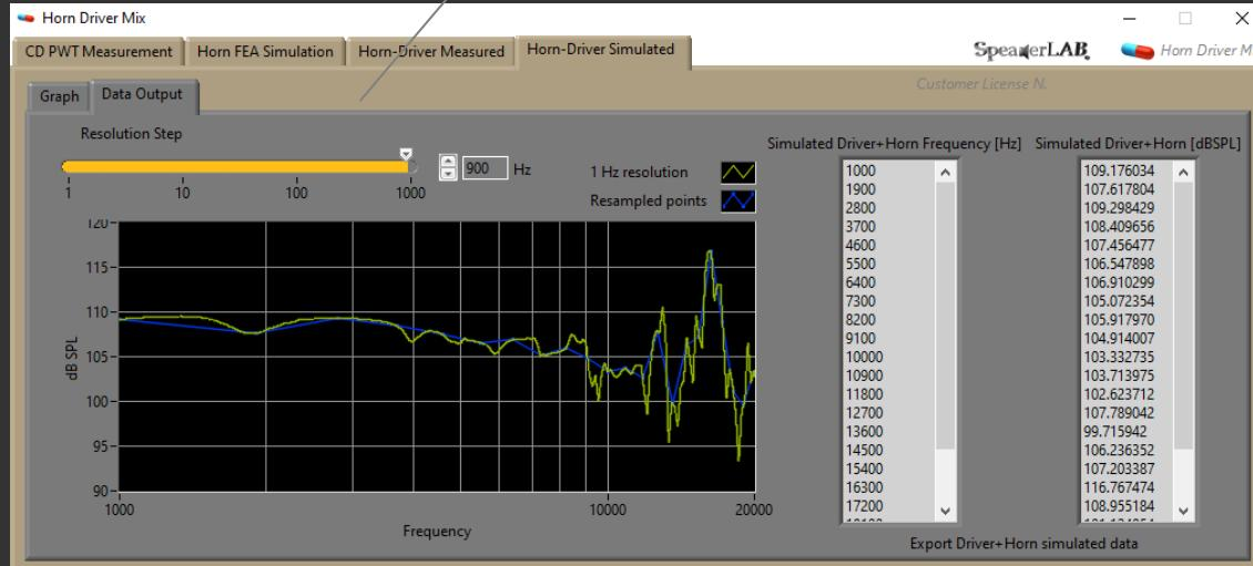
Copy Hz and dB SPL columns into your spreadsheet or measurement system
