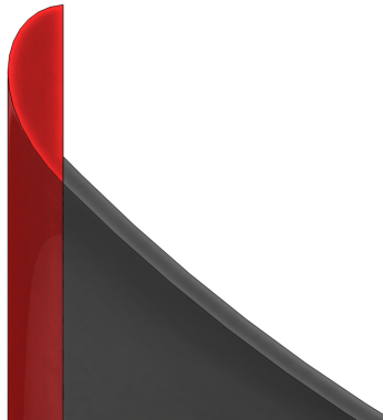
Figure 40. Example of a flared end, solid part in red, added to the exponential expansions horn mouth profile.
